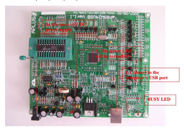
If the computer's USB ports are already connected to many USB devices, it will happen that the USB port does not have enough current output to drive the aP89W24USB programmer. In this situation, an external DC +6V power supply should be used instead of the USB.
