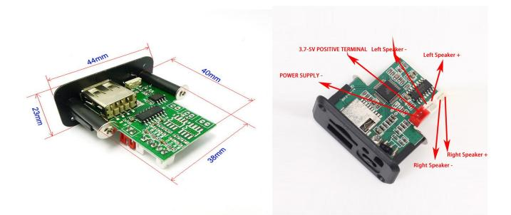
Power Supply: 3.7-5V lithium battery/5V adapter(Below 5.5V) The decoding board with 5V amplifier, apply with speaker directly Support WAV, MP3 FOMATE Supprt U disk & TF Card Support power memory
