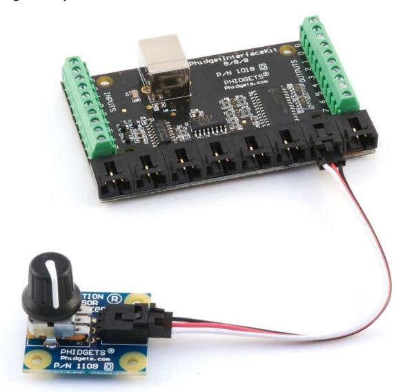
Connect the Rotation Sensor to an Analog Input on the PhidgetInterfaceKit 8/8/8 board using the sensor cable.
