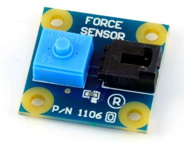
The Force Sensor is intended as a user input device (i.e recognizing that someone is pushing a button). It is not accurate enough to be used as a weight measurement device.
