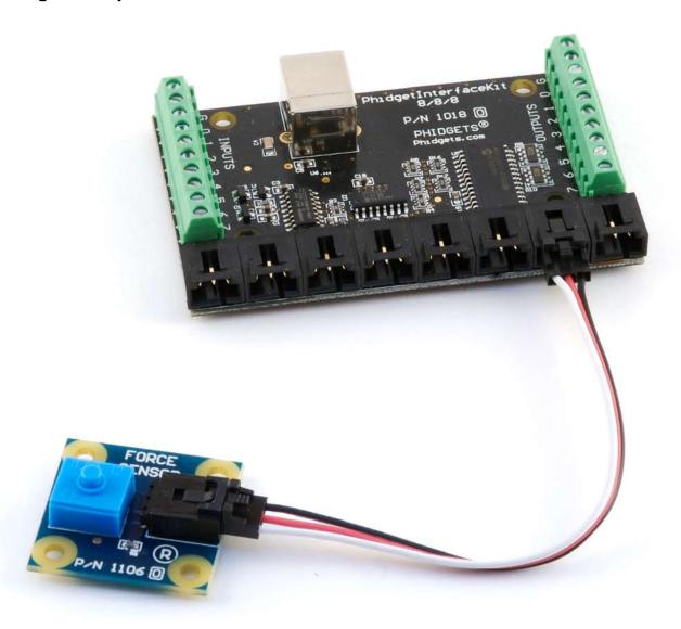
Connect the Force Sensor to an Analog Input on the PhidgetInterfaceKit 8/8/8 board using the sensor cable.
