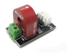
TA12-100 is a module for AC current measure. With 7 options, TA12-100 module has 7 sensitivities setting for much more application.
